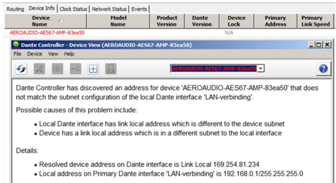
To change setting on the AMP you will need to match the IP address of the computer to the range of the AMP. In this case 169.254.81.xxx
