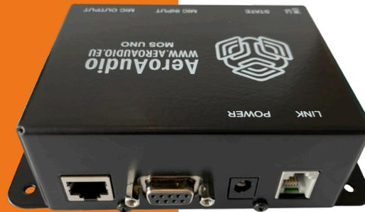
Suitable for signaling of on-air lamps for microphones. eg YELLOWTEC MIKA ON-AIR MIC ARM.
